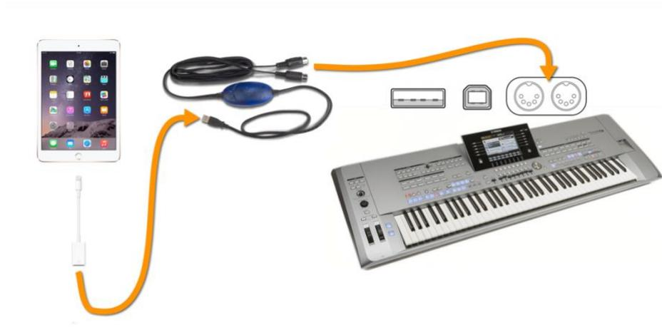
To avoid the adapter draining the iPad's battery, you can use an active USB Hub (with power supply) between the iPad and USB MIDI adapter.
