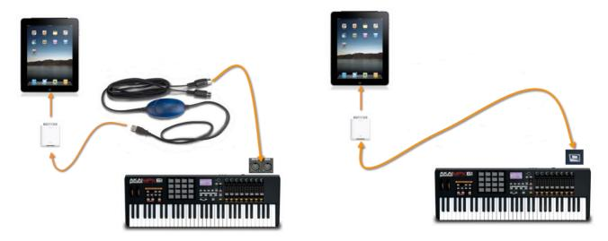
Attention: With the USB adapter connected, the iPad cannot be supplied with power at the same time!
